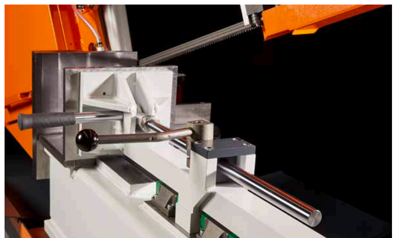
Material clamping by hydraulic short stroke vice.
