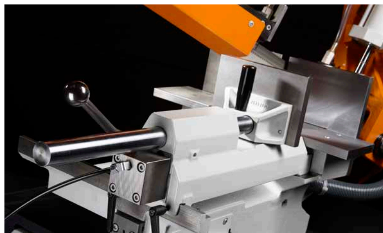
Material clamping by hydraulic short stroke vice. (U 2.6)
