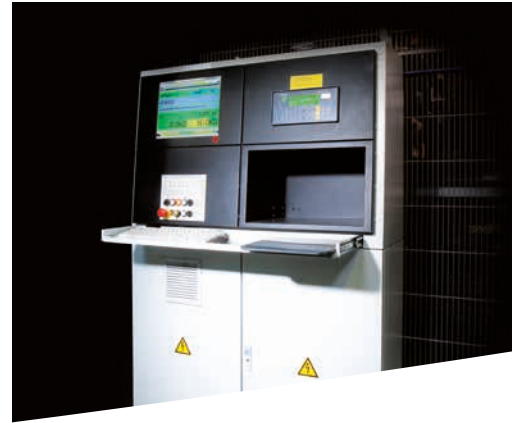
Easy operating by means of ergonomic operating panel with screen, keyboard, mouse, functions for manual operation and weighing device.
