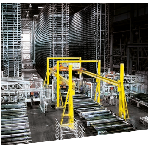
Largest commissioning storage system at a service center in the USA with fully automatic commissioning solution.
