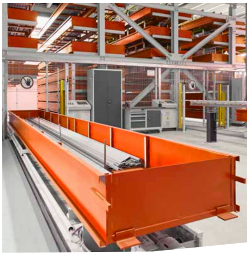
Longitudinal stations can be built-in at floor level or at any other height.
