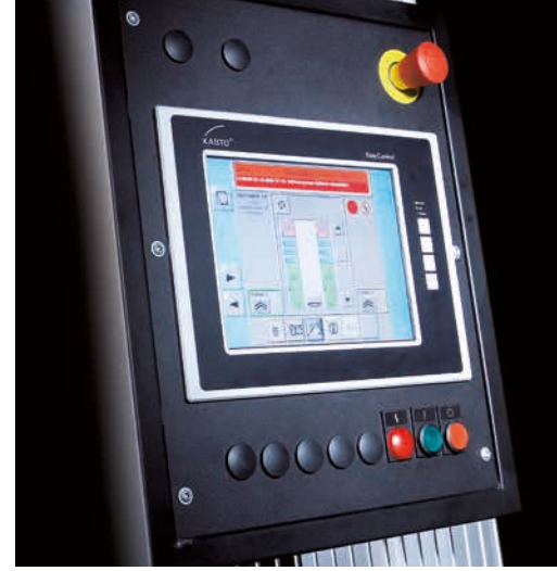
Operator-friendly control EasyControl , engineered to interface with customer's IT-System.
