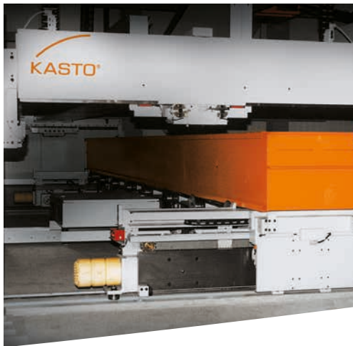
With an additional undercarriage, the UNITOP Bar Storage System is a fast commissioning system.
