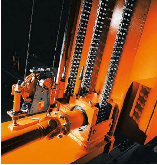
Durable and virtually maintenance-free: Operating Gantry Crane with chain hoist.
