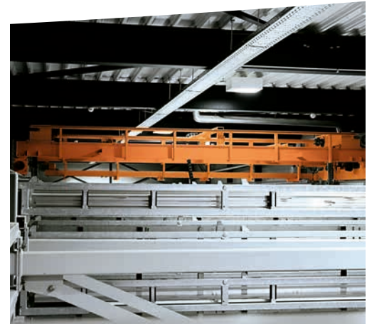
Overhead travel system for racks provided by the customer in window manufacturing.
