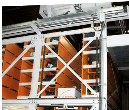
Overhead travel system UNITOP with tunnel for transport carriage.
