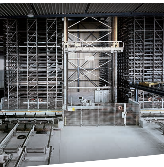
Commissioning storage system for bright steel and non-ferrous metals in service centers.
