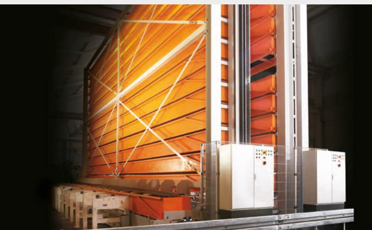
UNITOWER : Compact Cassette Storage System for bar stock, boxes and pallets.
