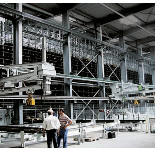
Commissioning device with magnetic system and chain conveyor for efficient commissioning.
