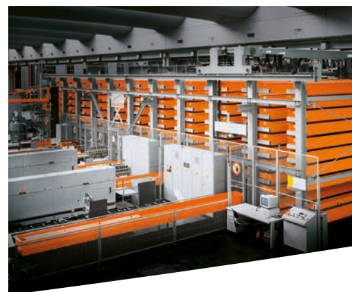
Overhead travel system UNITOP supplies different lathes and sawing machines.
