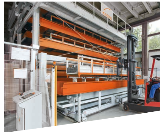
Loading station including integrated lining up and lifting device guarantees easy loading by fork lift.
